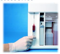
Easy sampling: Present a sample to the sipper tube and press the keypad. The 2300 automatically aspirates the sample and, in less than 60 seconds, displays and prints glucose and lactate levels.
